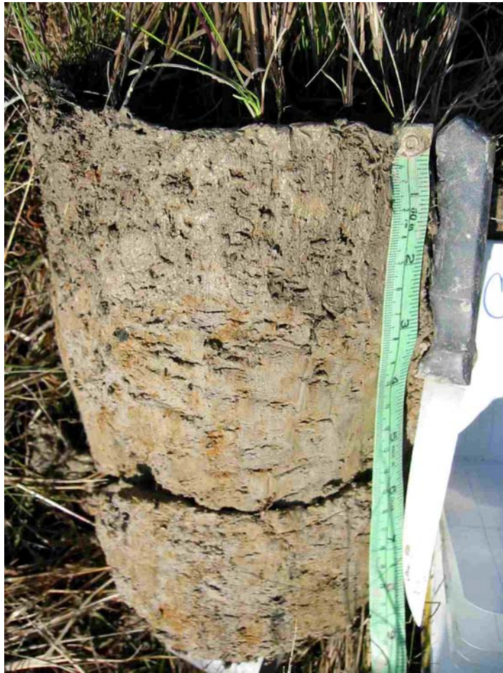
Figure 9. Intact soil block that has been excavated from a created wetland site per procedures outline in protocol. Note that the surface still needs to be “picked down” with a knife point to better reveal structure, redox feature location/size/abundance and rooting relationships.
