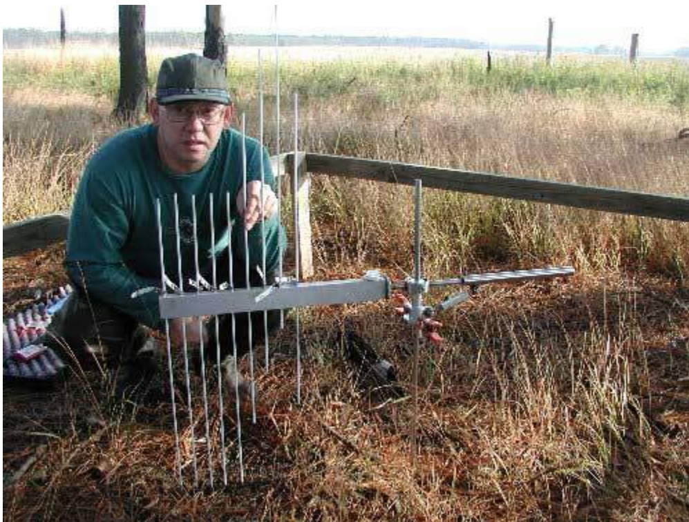
Figure 12. Reading the Rod SET at Blackwater National Wildlife Refuge. (Photo from the USGS Surface Elevation Table website at http://www.pwrc.usgs.gov/set/readSET.html .)
