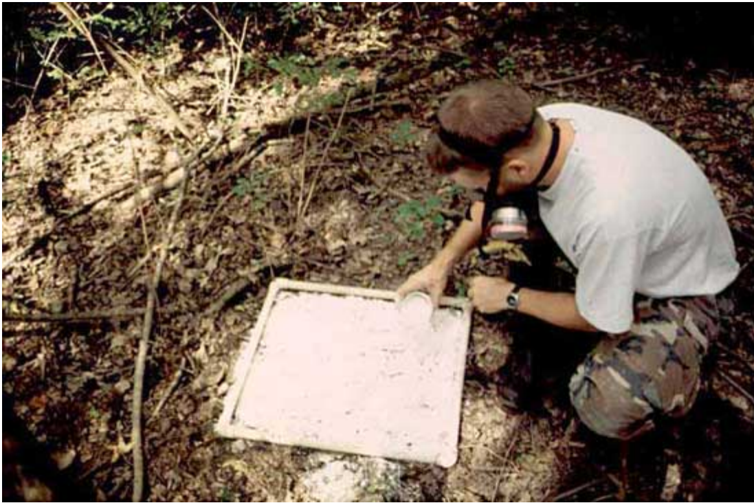
Figure 10. Installing a feldspar marker horizon in a forested wetland (photo is from the USGS Surface Elevation Table website at http://www.pwrc.usgs.gov/set/ )
